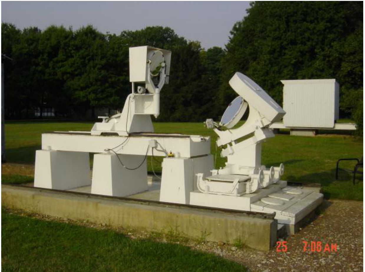
The cœlostæt that powers the 240mm objective and the objective (below)
